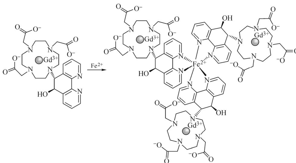
*Fig. 29.* Self-assembly of Gd-PhenHDO3A around  $\text{Fe}^{2+}$  resulting in relaxivity enhancement [ 13 ]
