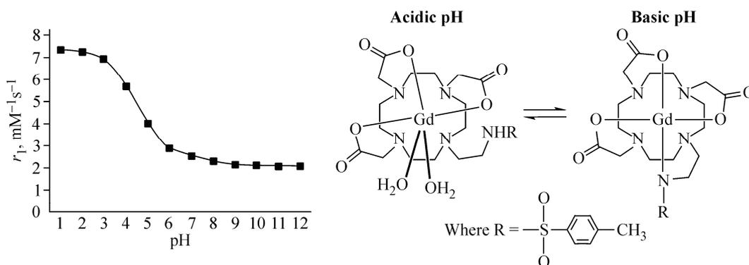
Fig. 15. pH dependence of the relaxivity of a Gd<sup>3+</sup> complex bearing an arylsulfonamide group. (20 MHz, 25 °C) [ 33 ]
