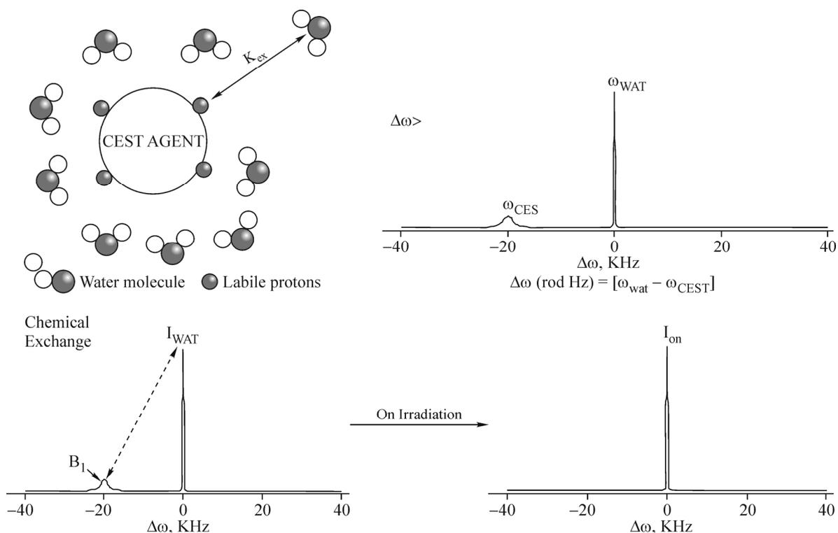
Fig. 30. Schematic representation of a CEST process [ 70 ]
