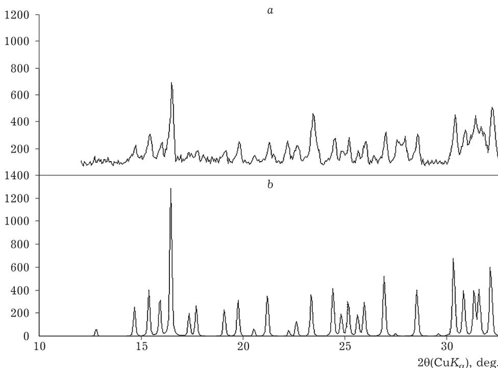
Fig. 2. XPA result of the crystallization product of the filtrate from drum 2 (a) in correlation with the the standard  $\text{Na}_2\text{S}_2\text{O}_3 \cdot 5\text{H}_2\text{O}$  (PDF 31-1325) (b).
