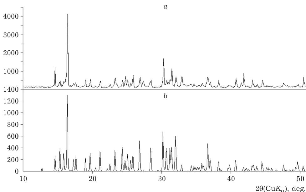
Fig. 1. XPA results of the crystallization product of the filtrate from drum 1 (*a*) in correlation with the standard  $\text{Na}_2\text{S}_2\text{O}_3 \cdot 5\text{H}_2\text{O}$  (PDF 31-1325) (*b*).
