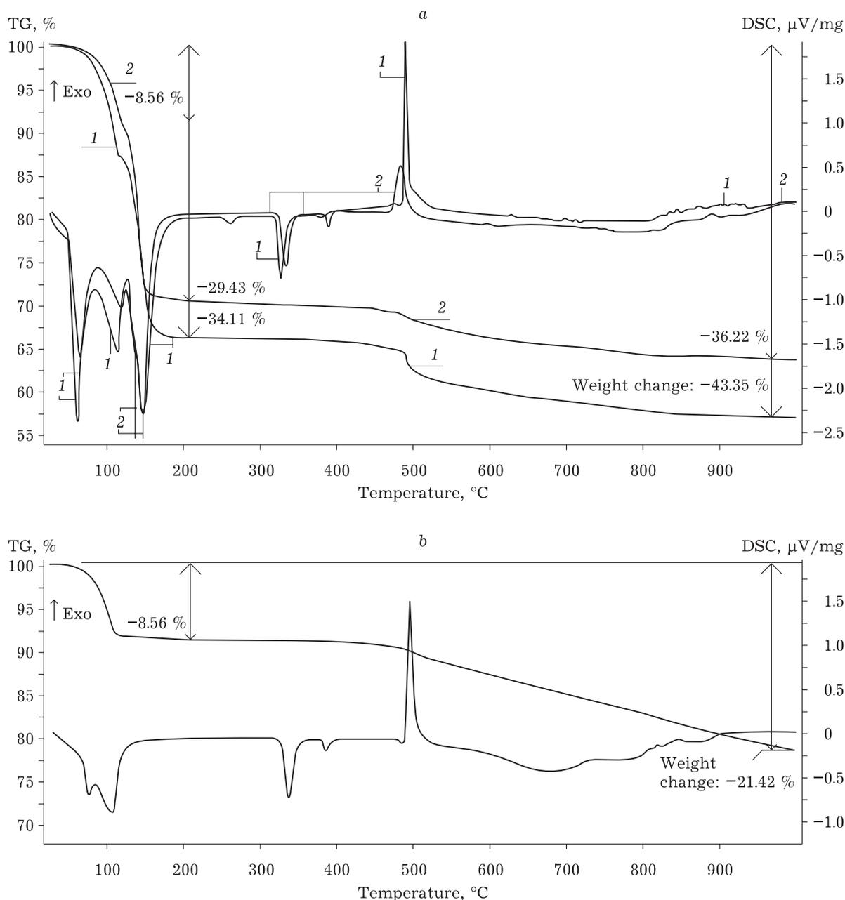
Fig. 3. TG/DSC curves of the samples of the solid phases: *a* – for reference pentahydrate  $\text{Na}_2\text{S}_2\text{O}_3 \cdot 5\text{H}_2\text{O}$  (1) and a sample from the filtrate of drum (1) corresponding to the composition of  $\text{Na}_2\text{S}_2\text{O}_3 \cdot 4.3\text{H}_2\text{O}$  (2); *b* – a sample from the filtrate of drum (2) (corresponding to the composition of  $\text{Na}_2\text{S}_2\text{O}_3 \cdot 1.3\text{H}_2\text{O}$ ).
