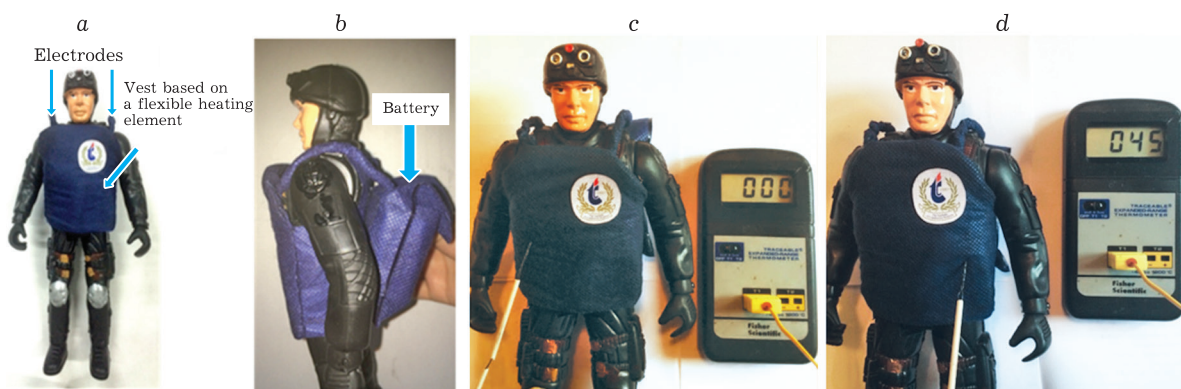
Fig. 8. Photographs of the maquette of a soldier (a, b) and the dynamics of changes of the vest temperature before switching it to the power supply (c) and after switching (d) [18].
