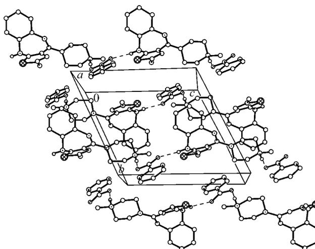
Fig. 3. Crystal packing viewed down a-axis. Dashed lines indicate N—H...O hydrogen bonds. H-atoms attached to C-atoms have been omitted for clarity
