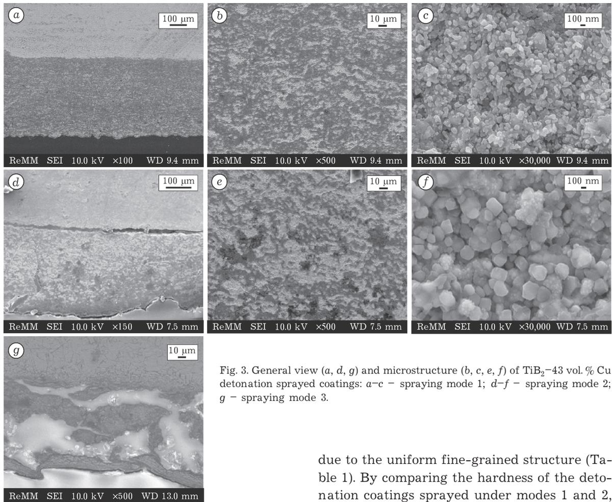
Fig. 3. General view (a, d, g) and microstructure (b, c, e, f) of  $\text{TiB}_2$ -43 vol. % Cu detonation sprayed coatings: a-c – spraying mode 1; d-f – spraying mode 2; g – spraying mode 3.
