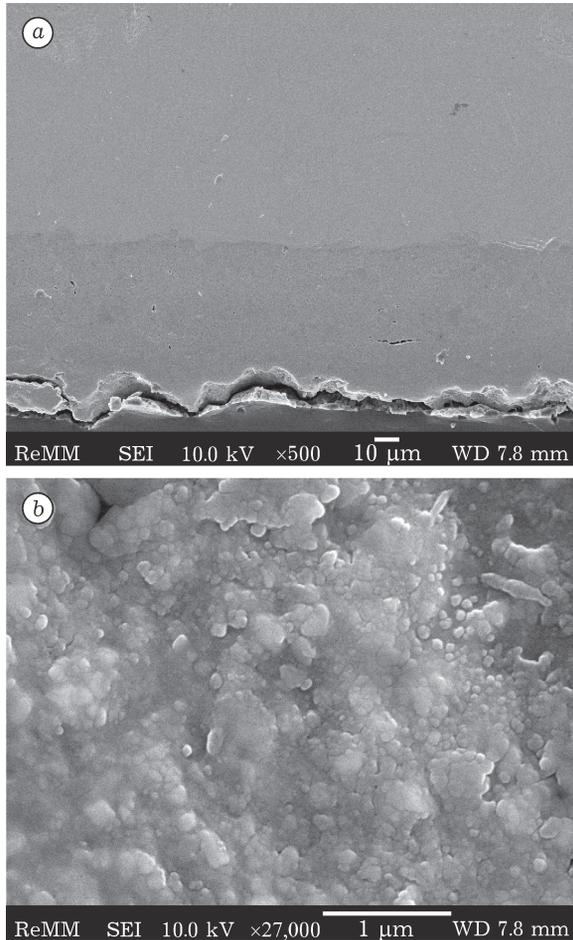
Fig. 1. General view (a) and microstructure (b) of TiB<sub>2</sub>-43 vol. % Cu cold sprayed coating.
