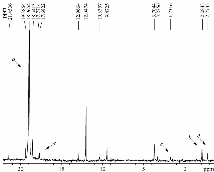
Fig. 3.  $^{31}\text{P}$  NMR: (a) trichlorfon, (b) dichlorvos, (c) methyl dihydrogen phosphate, (d) 2,2-dichlorovinyl methyl hydrogen phosphate, (e) methyl hydrogen 2,2,2-trichloro-1-hydroxyethyl phosphonate
