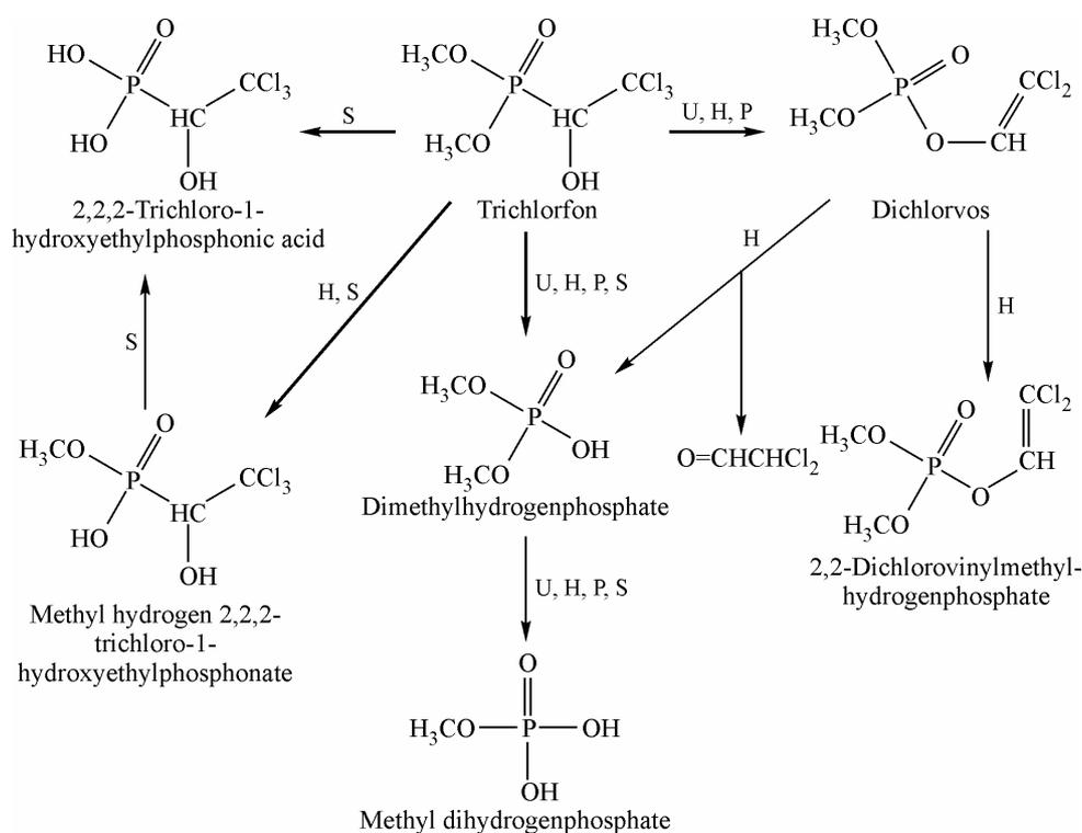
Fig. 1. Proposed degradation pathways for trichlorfon in the environment. Photolysis (U); hydrolysis (H); solid and microorganisms (S); plants (P)
