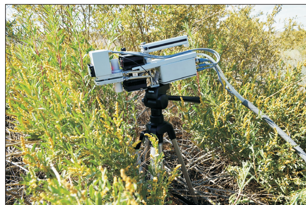
Fig. 2. Gas exchange measurements of four-winged saltbush in the field of Konya Karapınar.
