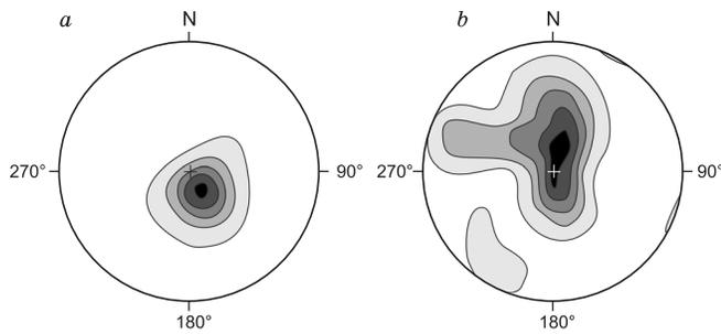
**Fig. 5.** Orientations of young low-angle zones of brecciation and cataclasis in the Sharyzhalgai uplift from the source of Angara to Kultuk community (a) and contacts of the Angara thrust (b). a, 153 measurements, contour lines  $> 4 > 8 > 12 > 15 > 20\%$  Wulff net, lower hemisphere; b, 177 measurements, contour lines  $> 3 > 7 > 12 > 15 > 18 > 20\%$ , Wulff net, lower hemisphere.
