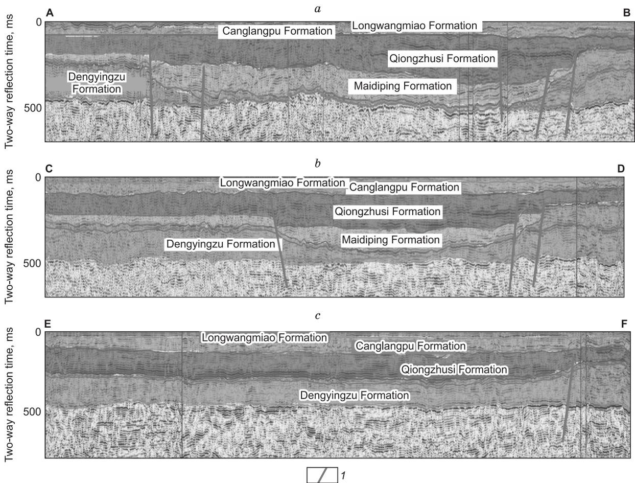
**Fig. 3.** Interpretation of the seismic section crossing the intracratonic rift (layer flattening by reflection top of the Canglangpu Formation, location see Fig. 2). 1, fault.
