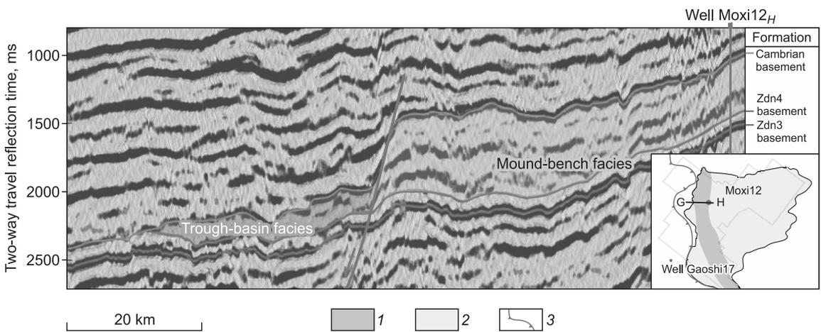
**Fig. 12. Seismic section of the trough basin and platform marginal mounds and shoals beside the intracratonic rift of the Dengying Formation.**
